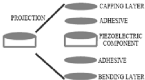
Fig 2: Structure of Piezoelectric component
